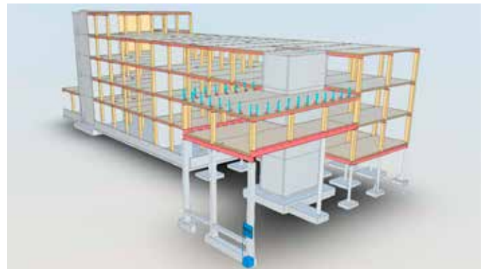
Modélisation BIM – design for disassembly, circularity profile and potentiel de remploi ©4D architects
